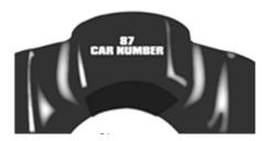
**4.5.3.7. Tub** - The Car number and Driver's first and last name must be 1 inch tall each. Letters and numbers must be in Impact font, black or white in color and no trim is permitted. This must be located directly behind the headrest. (See Illustration).
